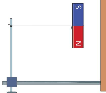
A freely suspended magnet aligns itself in the north-south direction.
