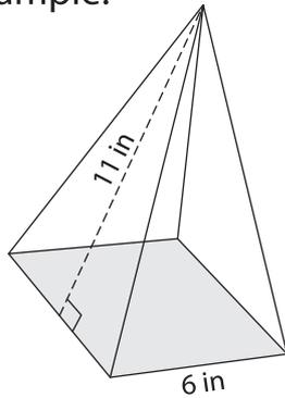
$$\text{Surface area} = \text{base area} + \frac{1}{2} \times \text{perimeter} \times \text{slant height}$$
